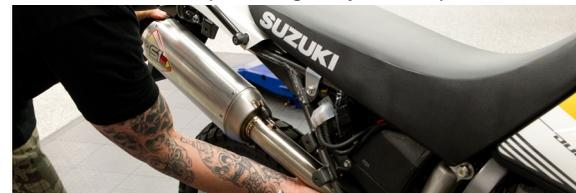
8. Install OEM bolt to mount TBR slip tube. Re-install OEM cover plate and tighten mounting bolts.
