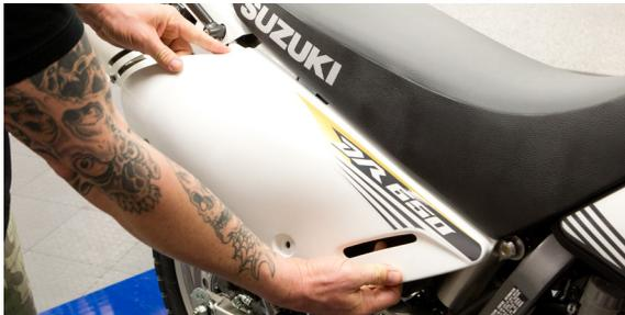
3. Remove plate to access joint clamp.
