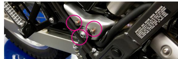
9. Slide muffler clamp over S1R muffler and attach to sub-frame using provided 55mm socket head bolt and spacer.
