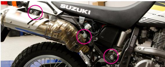
6. Attach slip-tube using provided hook springs.
