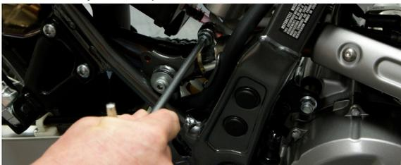
5. Remove three OEM mounting bolts. One bolt will be used with TBR system. Remove OEM muffler assembly.
