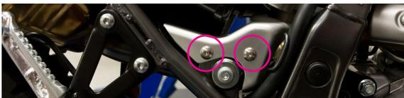
4. Loosen joint clamp.
