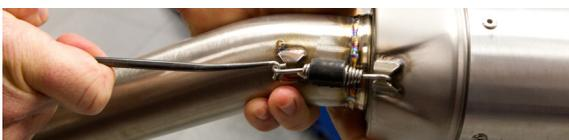
7. Slide TBR slip-tube into OEM header. OEM gasket will be used with TBR system. Tighten joint clamp.
