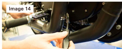
16. Before you run the bike, clean off all fingerprints and dirt, as any oily residue will etch the metal and become somewhat permanent when the system gets hot. Run the bike and enjoy. It is normal for some white smoke to appear the first time you start the bike. This is packing/manufacturing oil from inside the pipe burning off. Check for gaps or leaks. If you find a leak, a little high temperature silicon sealant should fix it. After 50 to 100 miles, recheck all fasteners for tightness.
