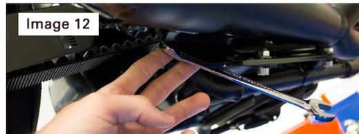
14. Once you ensure the exhaust clears the bike begin to tighten all hardware, starting from the header flanges and work your way back to the muffler. Install the included 45mm springs.
