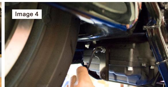
6. Now remove the OEM crossover and headers. Be careful to remove the O2 sensors as well.
