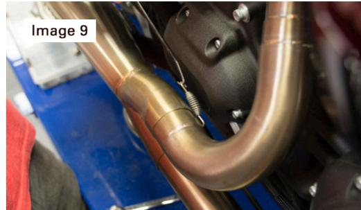
12. Now use the included 5/16" x 3/4" bolts to secure the muffler to the TBR bracket. The bolts will thread into the clip nuts you installed in step 11.
