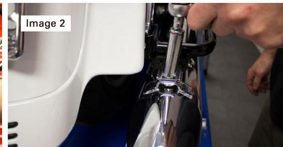
3. Remove the OEM mufflers and rubber mount brackets from the motorcycle.
