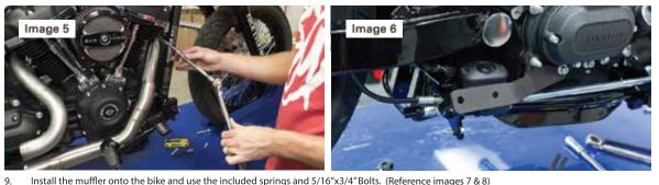
Install the muffler onto the bike and use the included springs and 5/16"x3/4" Bolts. (Reference images 7 & 8)
