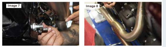
11. Now begin to tighten the headers and muffler to the muffler bracket. Start from the headers and work your way back to the muffler.
