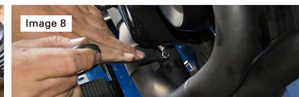
10. Tighten cylinder/header and muffler hardware to OEM torque specs.
