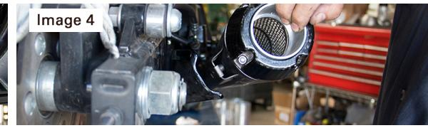
5. Attach muffler to both header pipes. (Reference image 3)
