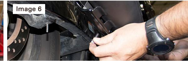
7. Line up holes on the bracket and frame for the supplied flange bolt. (Reference image 5)
