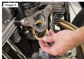
6. Now install the intake piece onto the backing plate using the suplied 1/4 - 20 screws and second gasket. The order of parts and gaskets should be as follows: Throttle Body, Gasket, Backing Plate, Gasket, Intake. (Reference Images 6 & 7)
