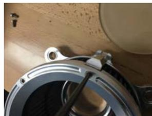
11. Install remaining 8/32 x 3/8" socket heads into the outer ring.
