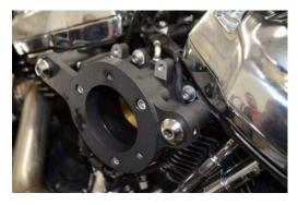
5. Install large O-ring onto backing plate and attach it to the offset adapter plate using supplied hardware (3  $\frac{1}{4}$ -20 x  $\frac{1}{2}$ ")
