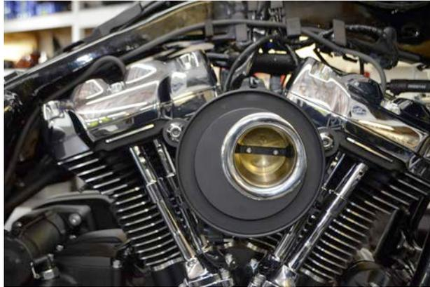
7. Install air cleaner element into backing plate.
