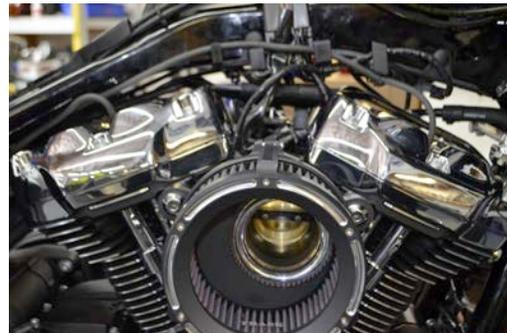
**NOTE:** If coating the raw air cleaner assembly, **DO NOT** coat the velocity stack . The magnets **CANNOT** be removed. Magnets are only removable from the backing plate with **EXTRA** care as to not damage the magnets. If damage occurs, they **CANNOT** be reused. In addition, any coating that requires a **HEAT** above 200°F will cause the magnets to **FAIL**.
