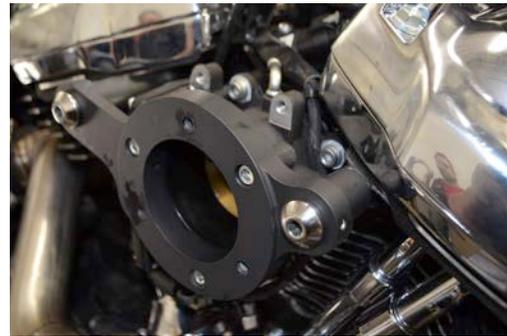
5. Install large O-ring onto backing plate and attach it to the offset adapter plate using supplied hardware (3 1/4-20 x 1/2")
