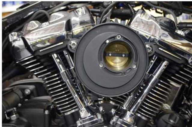
6. Install the velocity stack into the backing plate aligning magnets (it should snap into place)
