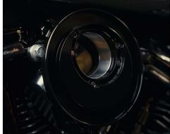
7. Install the velocity stack into the backing plate aligning magnets (it should snap into place).
