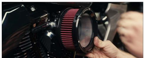
11. Install the 3 arms starting by hooking the pin behind the backing plate and rotating the arm into the slot on the outer ring.
