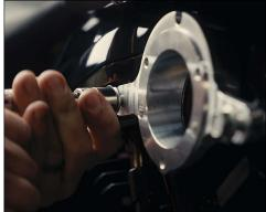
6. Install the air cleaner backing plate using three 1/4 - 20 fasteners.
