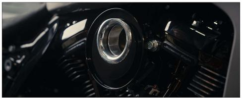
8. Install air cleaner element onto the backing plate.
