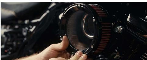
12. Torque the stainless cap screws to spec, securing the bezel to the air cleaner.
