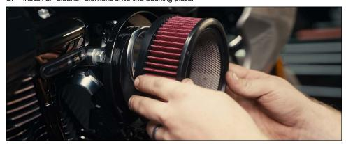
NOTE: Clock the air cleaner element so that the seam is on the bottom side.
