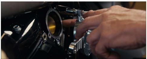
5. Apply red Loctite to the provided 3/8 fasteners that hold the sub-plate to the heads and torque to spec.
