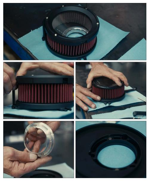
NOTE: The velocity stack is secured by magnets—two on the stack and two on the backing plate. Do NOT coat the velocity stack; the magnets are irremovable. Use caution when removing magnets from the backing plate to avoid damage. Damaged magnets cannot be reused. Any coating process exceeding 200°F will cause magnet failure.
