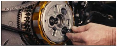
4. Place the Power Plate on top of the springs, ensuring each spring aligns with its seat on the reverse side.
