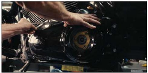
After installing the covers, be sure to refill the primary oil to factory specifications. Trask recommends BelRay primary-specific oil, Drag part number 3604-0003.
