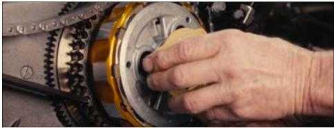
5. Install the three 12-point titanium bolts that hold the Power Plate in place. Tighten the three bolts evenly to prevent excessive pressure on any individual lug and torque them to 120 in. lbs.
