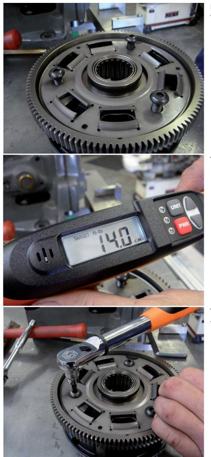
Be sure the plate is facing the correct way. You can now torque the plate down.
