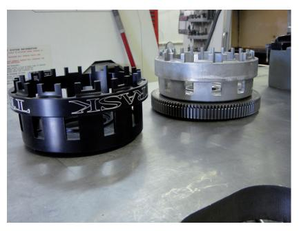
The Trask Billet Clutch Basket for 2002 to present. \*Note: We Highly recommend you use the model specific Harley manual for your bike to remove and install the clutch basket. The following instructions are for the the Trask Clutch Basket only.
