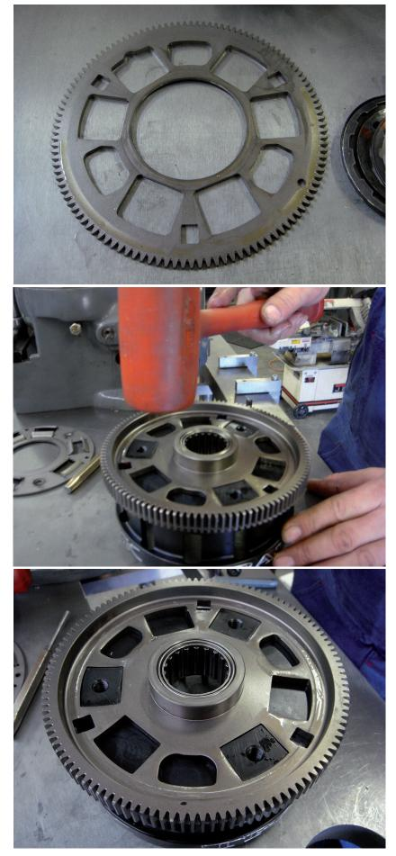
Remove and discard the back lash gear between the pinion gear and clutch basket.
