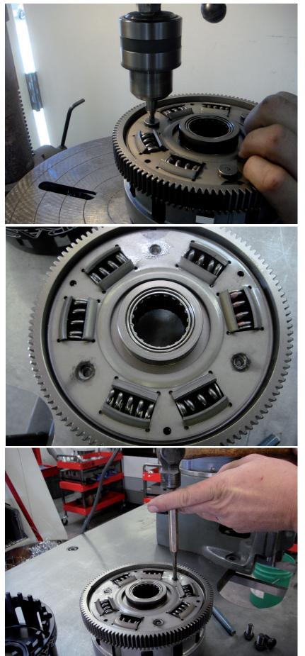
Using a 13/32 drill, drill out the head of the rivet but DO NOT drill all the way through.
