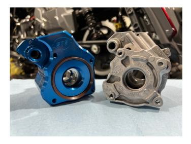
Please note the difference between the oil pump unit with the seal provision (LEFT) and the oil pump unit lacking the seal provision (RIGHT).
