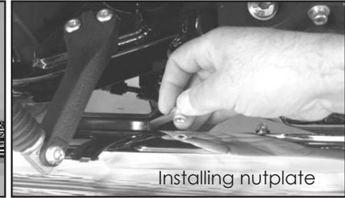
1. Attach mounting bracket 390-P to transmission and tighten to 12-15 Ft/Lb torque. (Figure 1). NOTE: 2006 to 2007 models use three 5/16" x 1-1/2" hex head bolts and washers. 2008 to 2009 models use three 5/16" x 1-1/2" hex head bolt, washers, 11/16" spacer between the bracket and transmission in top hole.
