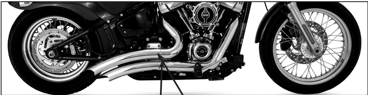
Check for good alignment at the seam
