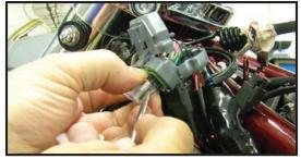
3. Locate pins 20 and 16 (unused in the current configuration), and remove the seal pin plugs. Insert the terminated black wire into pin 20, and the red wire into pin 16 on the "wire side" of the connector.
