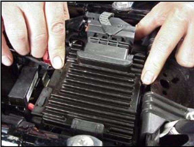
**FL-F:** Disconnect the ECM from the connector as per the following procedure: Depress button on socket housing of the connector; rotate locking bar until it reaches the full rearward position (the index pin on locking bar will engage the rear notch in the socket housing).
