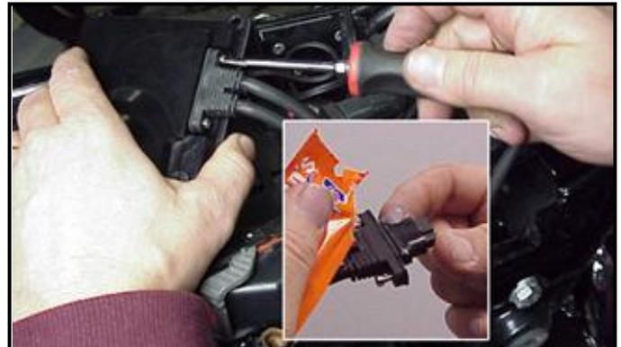
ECM. Before installing connector, lightly spread some dielectric grease on harness connector terminals, and on the inside lip of the connector port opening of the ECM to allow the rubber weather seal in the connector plug to slide into place without binding. Apply a dab of grease to the (2) upper and lower locating pins on the ThunderMax housing as well (arrows). See 'Tips' on page 7 for additional dielectric grease instructions.
