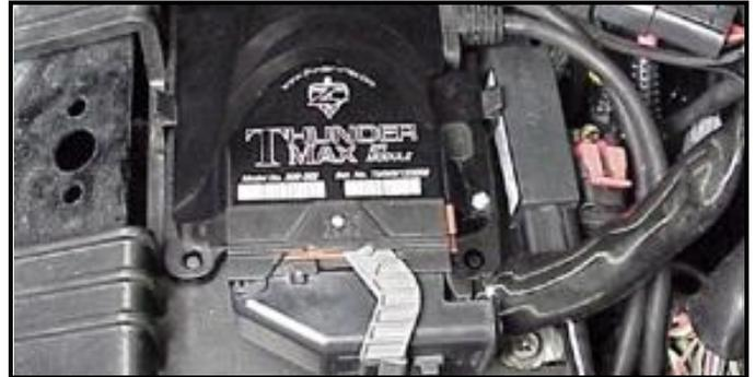
**FL-L:** Connect the oxygen sensor harnesses to the AutoTune harness. Carefully wire tie the leads to the motorcycle. Take extra care to ensure harness and sensor leads are safe from rubbing or chaffing on the motorcycle. Use all supplied wire ties; add extra ties if needed to properly secure wiring on your installation.
