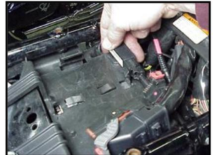
**FL-I:** Locate the package of dielectric grease included with communication cable. Spread a small amount of grease on the AutoTune harness plug inboard of the mounting flange to allow the plug to easily slide into the ThunderMax ECM, with ThunderMax logo on harness plug facing up. Attach with screws provided.
