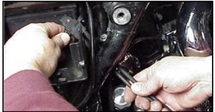
**FL-H:** If equipped with factory alarm, detach alarm antenna from ECM caddy clip by lifting slightly and sliding to the right of bike (do not disconnect).
