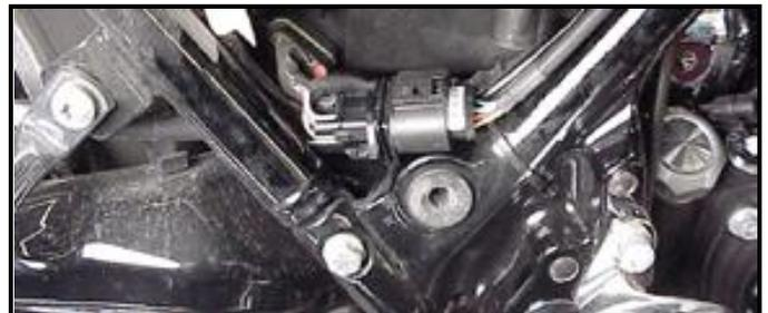
**FL-N:** Position front connector above lower frame rail between engine and transmission. Attach to existing harness with provided wire ties. Inspect all wiring to make sure it is clear of moving parts and excessive heat.
