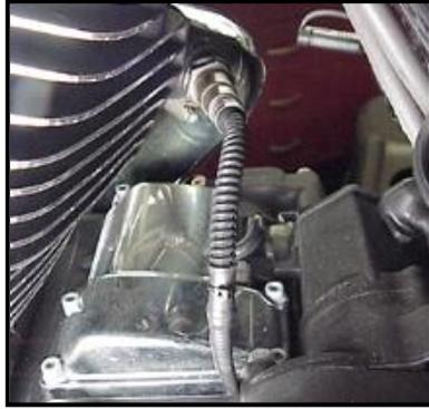
**FL-E:** Remove factory ECM from the caddy by spreading the plastic caddy latches at the sides of the ECM. Lift the ECM up and to the right to release it from the caddy.
