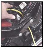
provided dielectric grease to the inside lip of the ThunderMax ECM to ensure the rubber weather seal does not bind upon installation, and across the pin casing on both 18 pin ECM connectors. Spread the grease across all of the female terminal openings, making sure the grease penetrates openings. This grease will help to maintain vital conductivity between the ThunderMax and the 18 pin connectors.
