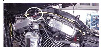
FXD-H: You will have excess harness on the rear sensor; gently bundle it together with a wire tie, connect it to the harness and tie it away from the engine and exhaust into the cavity between the battery and ECM caddy. After checking that all harnesses are securely tied down (away from any sharp edges that could chaff or cut harnesses), re-install the, gas tank, fuel line and seat. Re-install the maxi-fuse.
