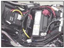
attach the fuse box to the plastic fuse box bracket.
