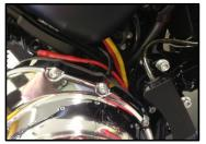
frame, loop the sensor and harness over the footpeg bracket towards the rear of the bike.
