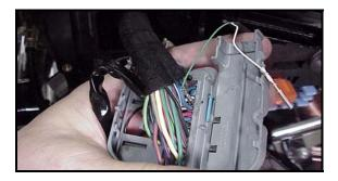
**4.** Locate the black wire in port #10 (redundant ground wire in the stock harness). Remove the pin & wire from #10. Insert the pigtail's terminated black wire into pin 10 on the "wire side" of the connecter. Pull the stock harness's wire back to cover with provided heat shrink and tuck into wire loom.
