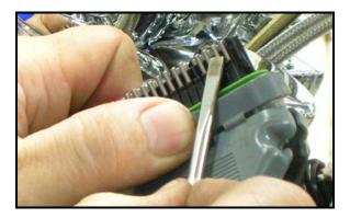
**6.** Re-install the connector retainer. Position the wires of the pigtail harness so that they exit the strain relief along the same path as the OEM wires. Close the halves of the strain relief around all wires.
