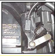
ThunderMax ECM connection port located under the retainer plate (loosen retainer screw, rotate retainer plate and open rubber weather seal). Open the TMaxII Tuner software and turn the bike's ignition and handlebar switches to the on/run positions. Follow the prompt instructions for installing the driver.
