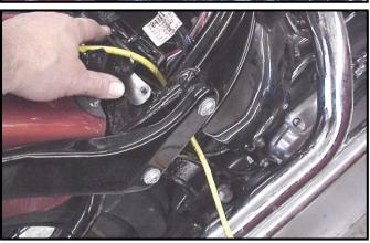
**FX/FLST-G:** Install the ThunderMax ECM onto the ECM caddy studs without nuts; insert the oxygen harness connector into the ECM with the imprinted "ThunderMax" logo facing up. Tighten the (2) Phillips connector screws. Lift ECM and install main 36-pin connector, ensuring it is fully seated and latched. Replace ECM onto studs.
