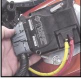
**FX/FLST-H:** Unplug and remove factory oxygen sensors from exhaust if equipped (rear sensor plug located under oil tank). Rubber caps are included to cap off the factory
