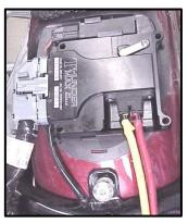
XL-D Route front the oxygen sensor lead along the left front frame tube to under the fuel tank shown. as Route the front ECM O<sub>2</sub> harness from
