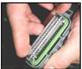
Also apply dielectric grease to the ThunderMax oxygen sensor harness connector terminals for improved conductivity, and to the outer housing to prevent binding upon installation to the ECM.
