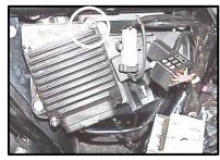
FL-C: Remove the factory ECM from the motorcycle, the ECM is held to the electrical caddy by socket head cap screws. The screws have a locking agent on them and can be difficult to remove.
