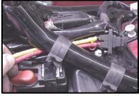
XL-B Remove the left side cover, locate and remove ECM the Power fuse. Remove the seat. unplug and remove the factory ECM. Feed the ThunderMax oxygen
