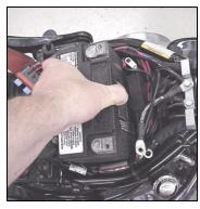
**FX/FLST-C:** Remove the (4) mounting nuts holding the factory ECM in place and lift the ECM from the mounting bracket. Depress the latch on the main connector and remove the factory ECM from the wiring harness.
