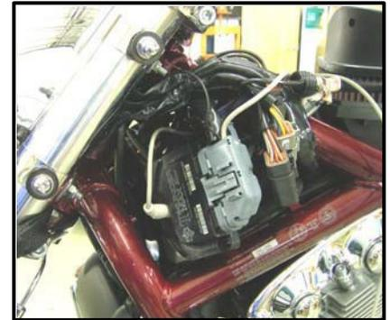
Once option 1 or 2 is performed, install the ThunderMax ECM to the motorcycle in the stock location. Plug the main harness into the ECM and reinstall the ECM fuse.
