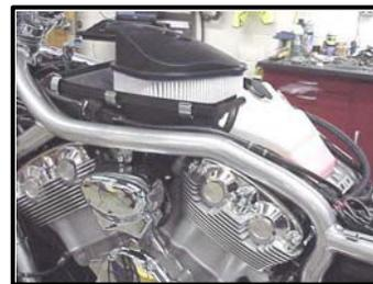
Route the harness along the upper left frame rail and plug the oxygen sensor harness into the AutoTune harness plug marked "REAR". It is very important to install these correctly or the engine will perform
