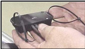
Loosely loop a wire tie through each slot in the supplied AutoTune module.
