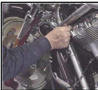
Route the oxygen sensor harness from the front pipe along the left frame downtube, across to the right side of the frame in front of the cylinder head cover, away from the engine and along the frame when possible.
