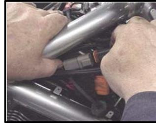
Plug the 4-pin AutoTune connector into the gray data port connector. It is through the data port that data from the AutoTune module is transferred to the ThunderMax.
