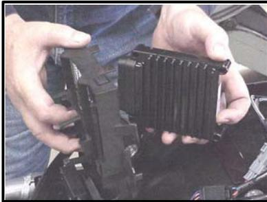
Locate and remove the ECM fuse. Unplug the ECM and remove the ECM with the plastic ECM caddy (unsnap the caddy from the fender). Separate the ECM from the caddy.
