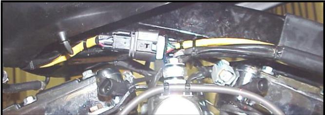
**FXD-H:** For the rear cylinder, connect the oxygen sensor; coil and tie the excess harness and locate it in the pocket behind the ECM caddy in front of the frame backbone.
