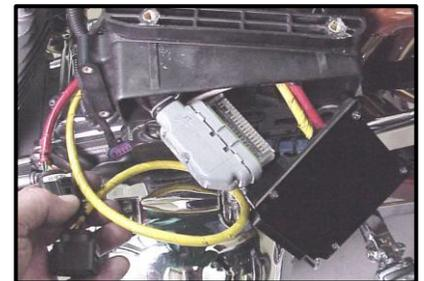
**FXD-F:** Reattach the caddy to the chassis with the two top frame bolts, taking care not to pinch any harnesses behind it in the process. Connect the greased 36-pin ECM connector to the ThunderMax ECM. Route pigtail harness for convenient access under cover as shown.
