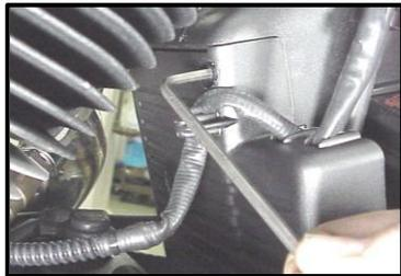
**XL-D:** Remove the stock ECM out of the caddy, towards the primary side of the motorcycle. Lift tang on the top of the caddy to help release the unit.
