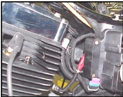
**FXD-I:** Securely tie all harnesses to the frame and/or other harnesses with supplied wire ties. Avoid sharp turns while routing harnesses and avoid areas where engine movement, sharp edges, exhaust systems or hot engine components can contact and cut into the harnesses or connector plugs. **Re-install the ECM fuse,** ignition coil assembly, gas tank, fuel line and seat. Advance to step 3.
