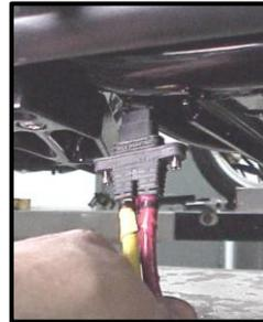
**XL-G:** Route the oxygen sensor harness into the ECM caddy. Starting from under the chassis between the rear engine mount and rear frame cross member, behind the belt, tight to the engine case. Feed the ECM plug between the bottom two oil tank hoses into
