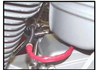
**ST-B:** Locate and remove the ECM fuse. Remove rear fender assembly and rear wheel to access ECM mounting caddy. Remove the plastic shield, then the ECM caddy mounting bolts.
