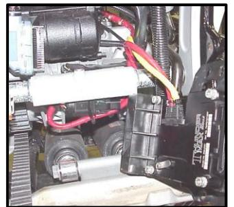
**ST-E:** Route the front sensor lead along the right frame rail, position connector as shown behind brake pedal.
