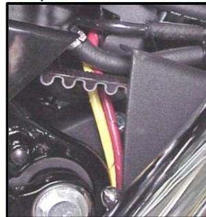
Connect the greased 36-pin ECM connector to the ThunderMax ECM. Install the ThunderMax ECM into the ECM caddy while gently pulling the oxygen sensor harnesses down from under
