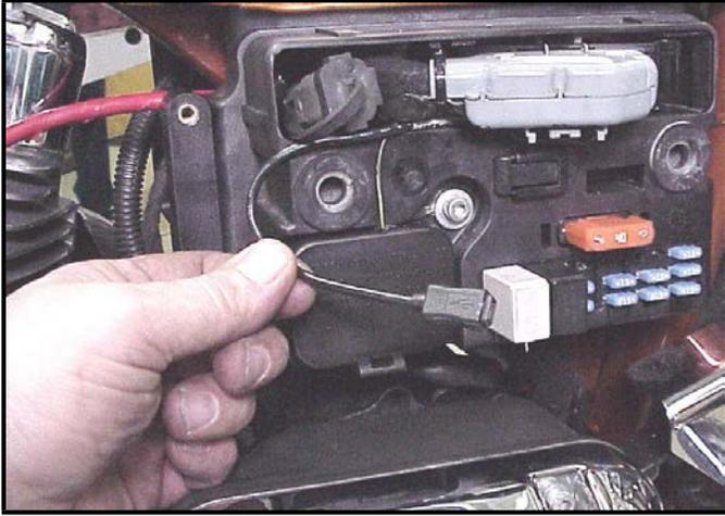
**FXD-G:** Route front ECM sensor lead along left frame backbone under gas tank; position sensor plug just forward of engine mount top link. Route front oxygen sensor lead up left frame tube to connector as shown. Check that connector position does not interfere with gas tank when in position before securing with wire ties.
