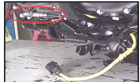
front cylinder towards the front of the engine between the left frame tube and the engine (a tight fit that may require some patience).
