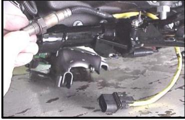
Install the rear sensor the same way, except once it's through the frame, loop the sensor and harness over the footpeg bracket towards the rear of the bike.
