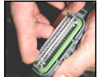
Also apply dielectric grease to the ThunderMax oxygen sensor harness connector terminals for improved conductivity, and to the outer housing to prevent binding upon installation to the ECM.
