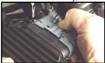
**XL-E:** Fully depress connector tab and disconnect the stock ECM from the 36 pin connector.
