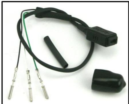
the left side of the motorcycle, between the module area and the frame back bone, coming out above the battery. Use a wire tie on the connector to the main harness
